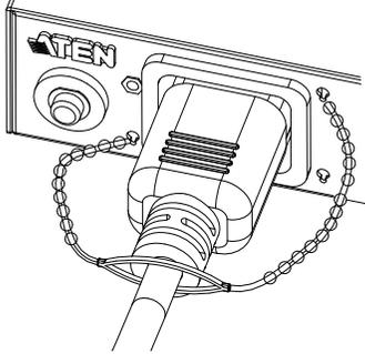
For EZ-Lok Plug Connectors fit the plug connector onto the input end of a C14 or C20 plug until it clicks in place and then connect the plug with the EZ-Lok Connector into the PDU by sliding it directly over and straight into the outlet.
